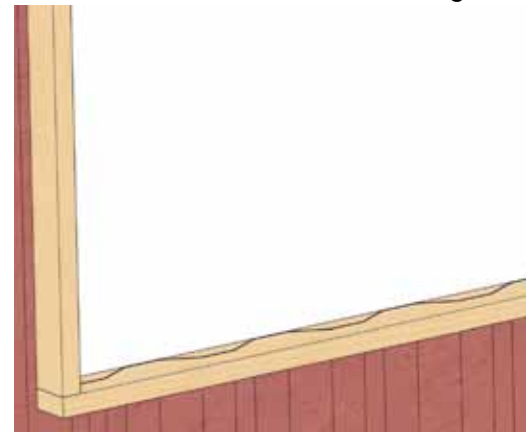
Wood jamb installed.
