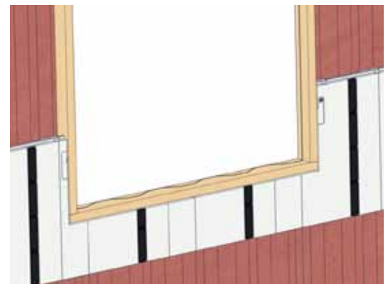
Leave a 1/4" gap for spray foam.
