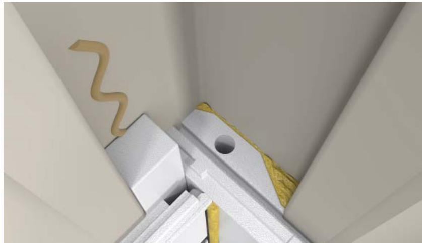
Fill the corner with foam.
