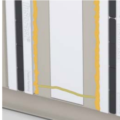
Omit spray foam at bottom for drainage.
