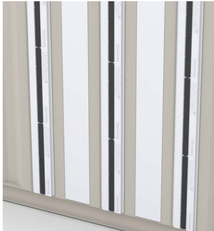
Install the Side Wall Inserts in the alternating corrugations.
