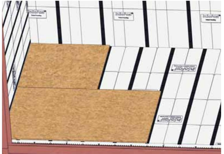
Make sure the long seam of the plywood does not line up with the InSoFast panels.
