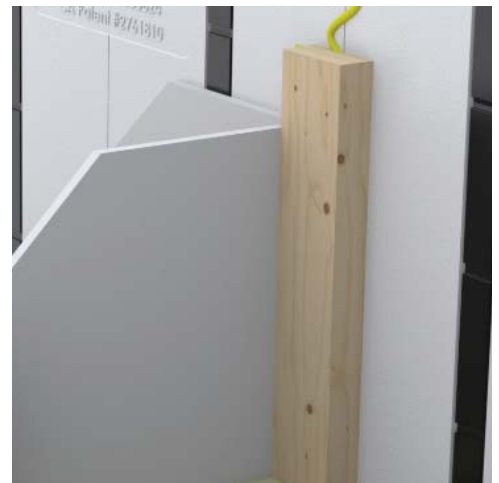
Interior wall glued to panels.
