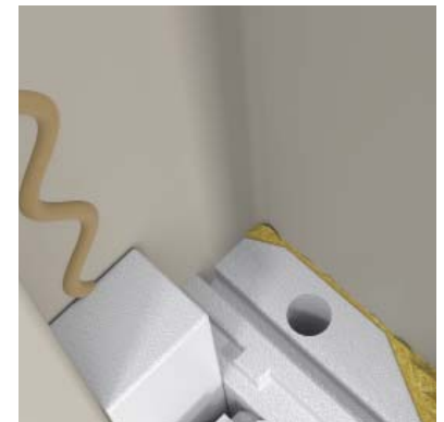
Fill the corner with foam.
