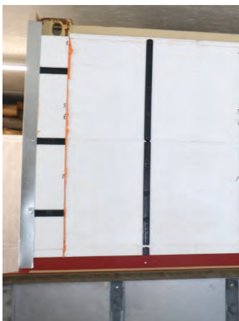
Metal flashing installed for added attachment.
