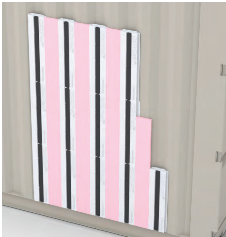
Use 5" wide sheet foam when LowPro is installed in every corrugation.
