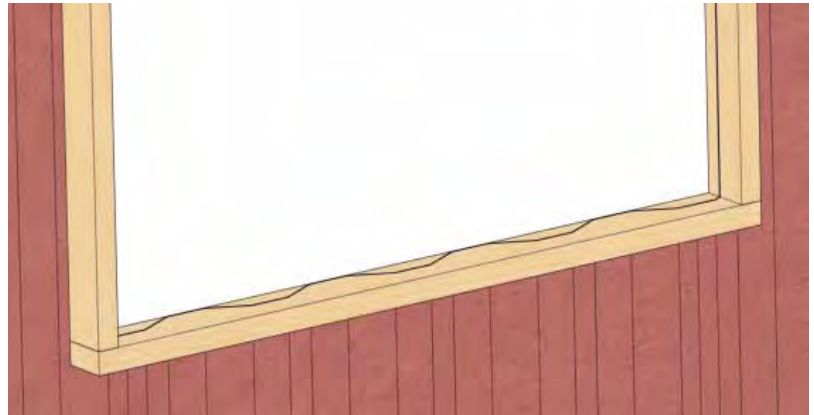
Wood jamb installed.
