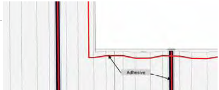
PL Premium on the studs and around the cut out. Spray foam on the top of the panel.
