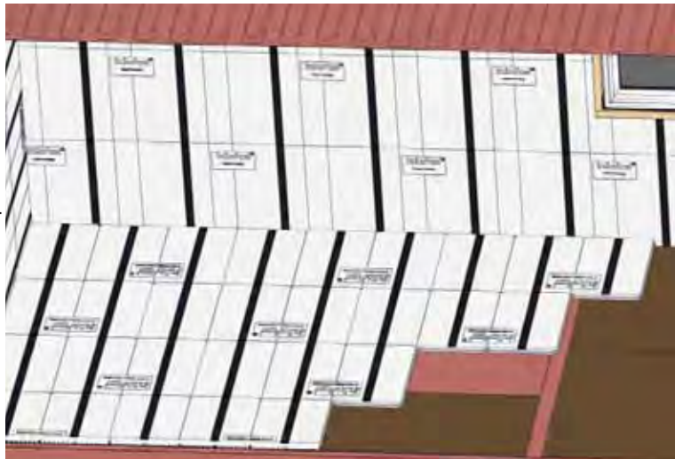
Install UX panels in a running bond pattern.
