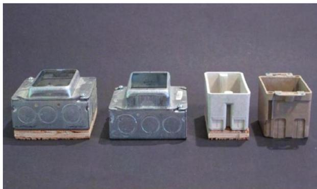
9. Install a 2-1/2" deep box, a 1 1/2" deep box with a 1" mud ring or a 2" deep box with a 1/2" mud ring. Secure plastic, metal, or fiberglass electrical boxes directly to the concrete wall with adhesive or a mechanical fastener.
