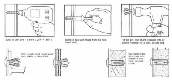
Note: If pin in rivet does not drive flush when fastening into solid materials and applications where expansion may be restricted, larger hole is required, use .261" - G bit.
