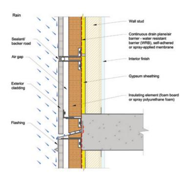
materials were backed by an air gap. Examples include wooden shingles on skip sheathing, masonry veneers and heavy masonry walls with 1- to 2-inch cavities separating brick walls and beveled siding installed shingle style. The air gap between the siding and the interior of the wall enables wet porous materials to dry out to either the outdoor air or into the air gap.
