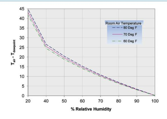
has to be  $3^{\circ}F$  cooler than the air for condensation to occur. It is very likely that during normal operation in many seasons there will be surfaces in buildings that are  $3^{\circ}F$  colder than room temperature.
