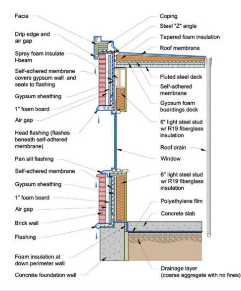
the importance of flashing that is both well designed and well installed. There are no certification programs for the proper installation of flashing; however, the following trade associations offer educational materials and training programs for flashing design and installation:
